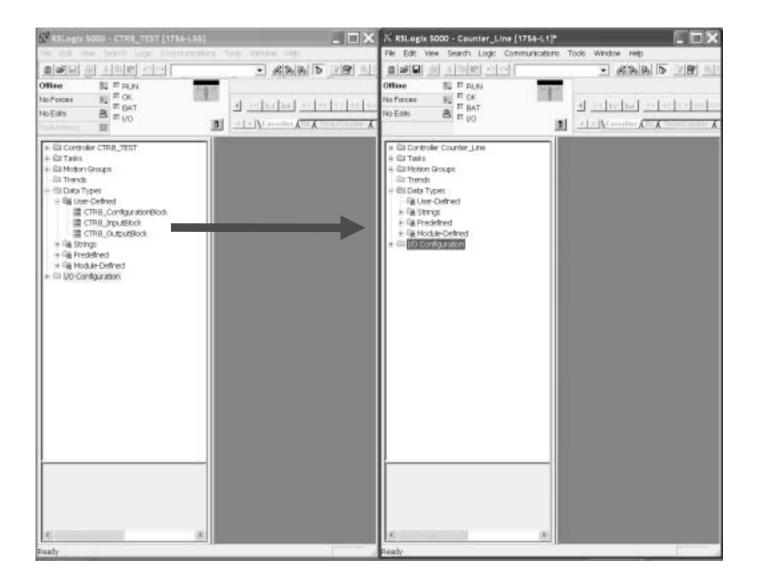
Step 3- Drag and drop the controller configuration tags from the sample project into your project.
