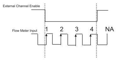
Given the above wave form, the module will begin counting the first positive going input pulse after the external enable input goes low. The module will accumulate 4 counts in the channel count register and stop when the external enable input goes high.
